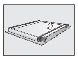
■ Refit the fibre-glass seal by feeding the ends back into the side fixings.
